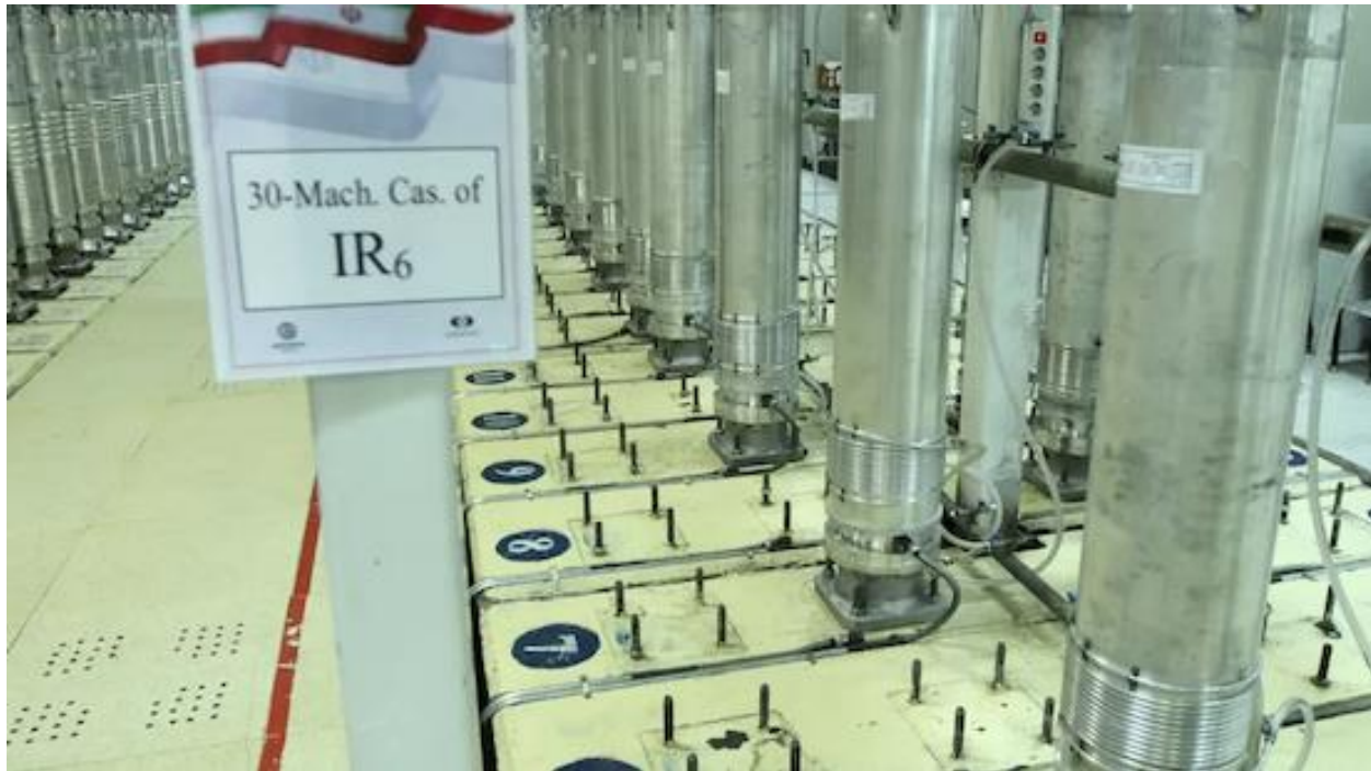
Advanced IR-6 centrifuges in the underground and hardened Natanz uranium-enrichment facility in central Iran. (Atomic Energy Organization of Iran)
